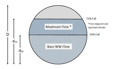
Figure 2. Gravity sewer assumptions for base wastewater flow (50% full) and capacity (75% full).
