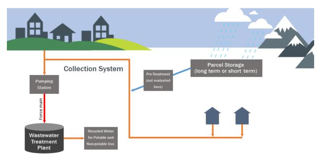
Figure 1. Stormwater capture concept for flow augmentation to sewer systems.
