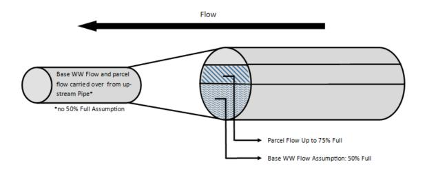
Figure 3. Assumptions for flow in gravity sewers when pipe diameter decreases going downstream.
